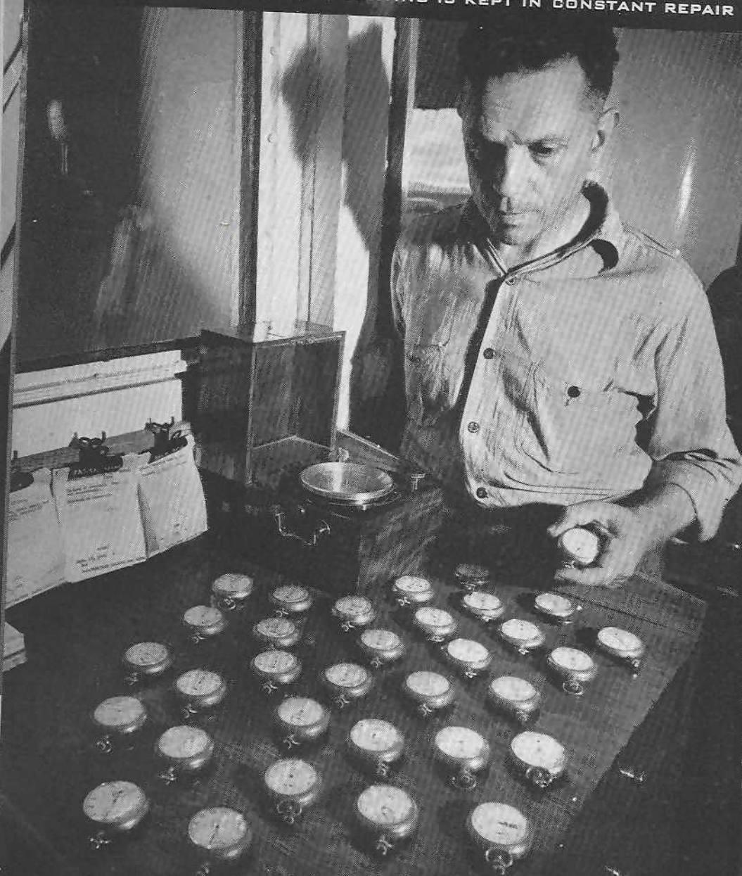
32 STOPWATCHES ARE CHECKED BY CHRONOMETER BEFORE USE
